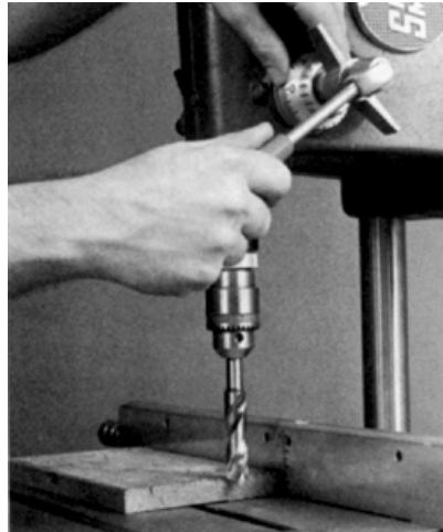
Figure 7-10. Use the depth control to keep the bit from biting through the scrap block and into the worktable.
