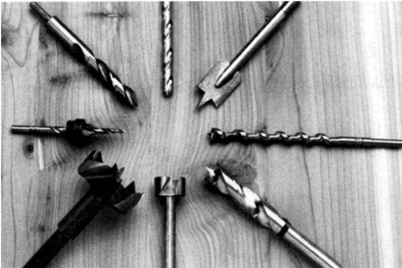
**Figure 7-3.** The most common types of drill bits are: (A) twist bits, (B) spade bits, and (C) power auger bits. Examples of specialized drill bits include: (D) brad-point bits, (E) Forstner bits (F) multispur bits, (G) screw bits, and (H) plastic-drill bits.
