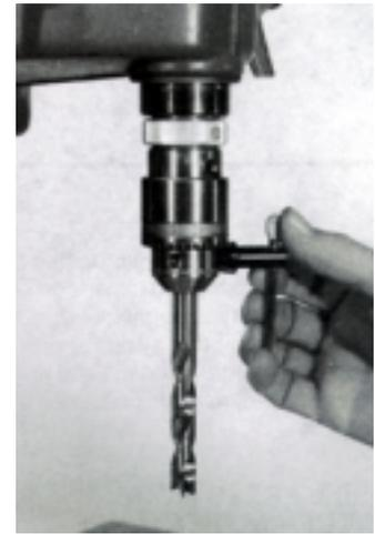
**Figure 7-4.** Drill bits are secured in the chuck with a special key.
