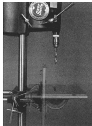
**Figure 7-2.** In the drill press mode, the table tilts from "0" to 90-degrees.
