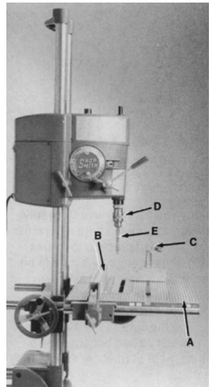
**Figure 7-1.** The accessories that are used for drilling operations are the (A) worktable, (B) rip fence, (C) miter gauge, (D) drill chuck and (E) drill bit.
